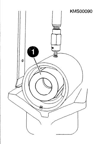
Replacing excitation winding
